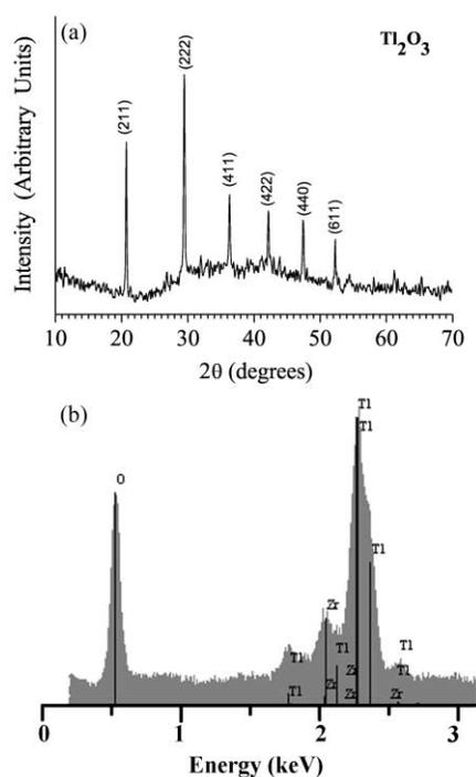
**Fig. 8** X-Ray diffraction pattern (a) and energy dispersive X-ray analysis (b) of a  $\text{Ti}_2\text{O}_3$  film deposited on random YSZ substrates ( $430^\circ\text{C}$ , 14 Torr) using the  $\text{Ti}(\text{hfa})_3$ -tetraglyme adduct.
